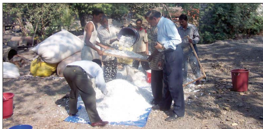
Screening of plastics waste to the required size
