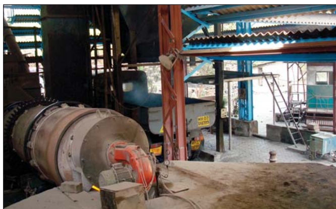
Rotor and mix discharge unit
