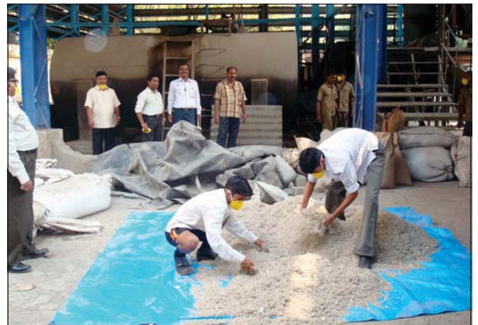
Plastics waste being prepared for mixing with the bitumen and aggregate
