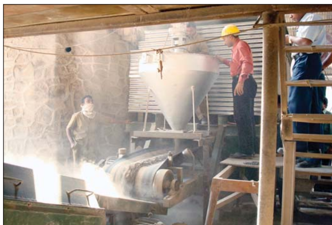
Plastics waste being added through automatic dosing machine
