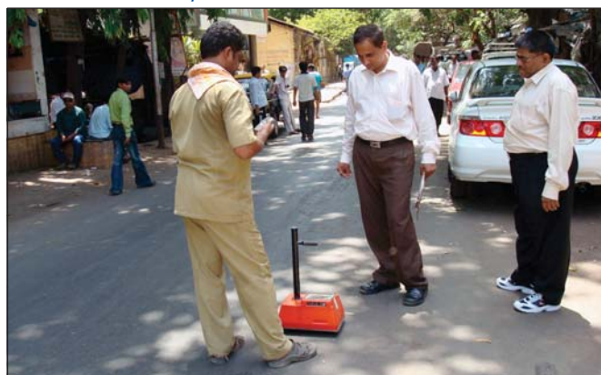
MCGM Road Testing Engineer is testing the density of the road using automatic Nuclear Testing Device.
