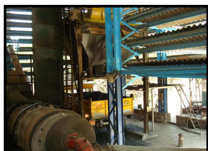
Plastic Coated Aggregates blended with bitumen being loaded on the transporting vehicle
