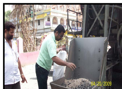
Shredded plastic waste being mixed with aggregates: Batch Process
