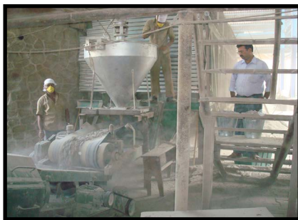
Shredded plastics being added from dosing device over the Aggregates on conveyer belt
