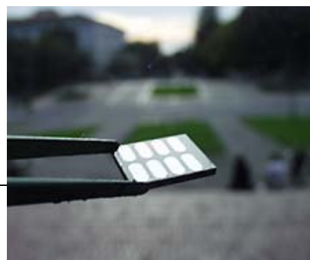
A panel of eight plastic solar cells based on inorganic nanorods and semiconducting polymers. The shiny ovals are the aluminum back electrodes of the individual solar cells.
